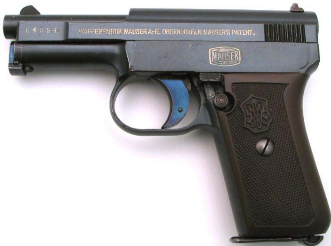
1910/14 transitional, Manufactured from 1914 to 1921, serial number range 61000-221800 (no latch in side plate, 9 slide serrations)
