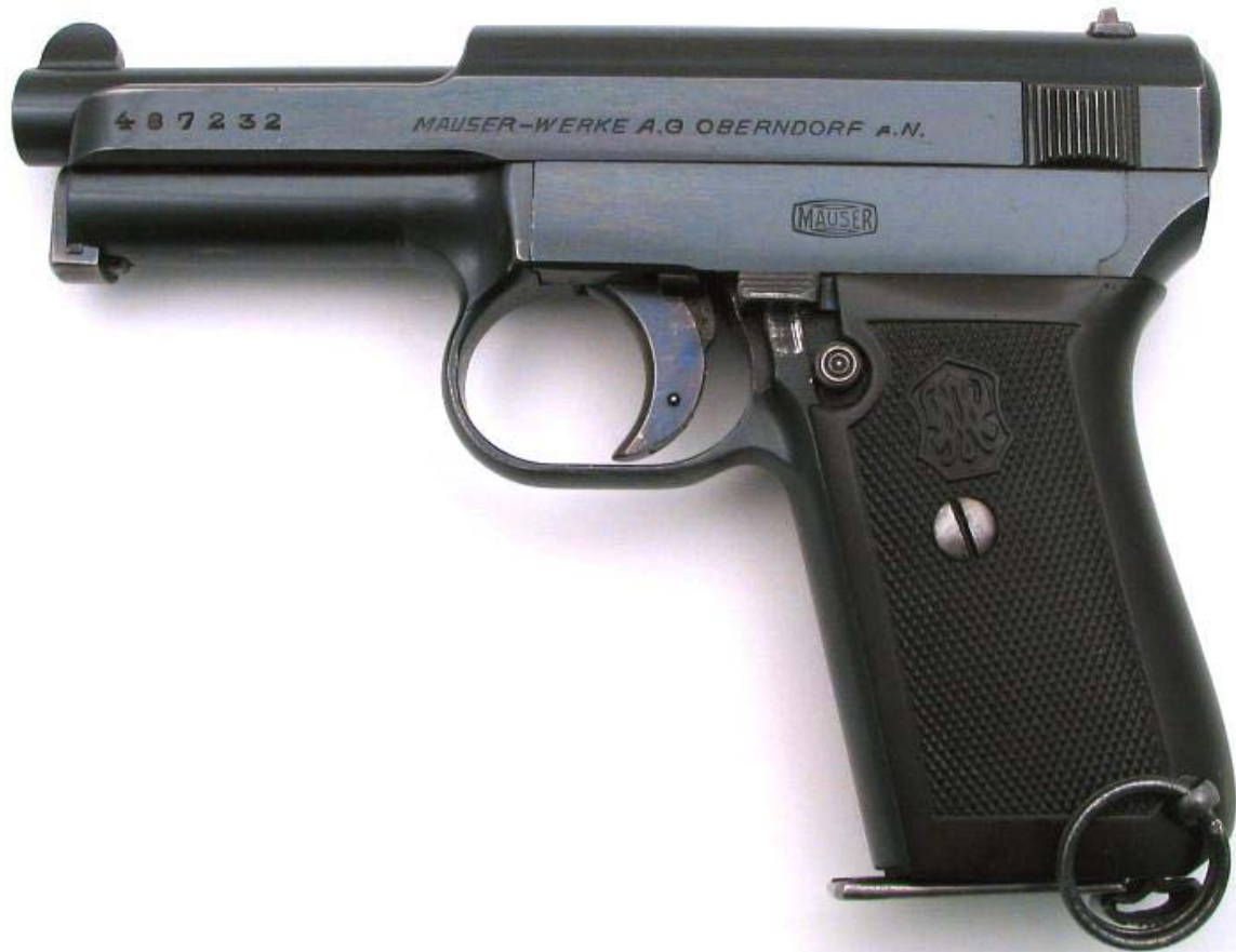
1914/34 transitional, Manufactured from 1929 to 1933, serial number range 460000 - 526000 (Mauser Werke address, straight grip, finish changed from cold blue w/small parts nitrate blue to hot dip, later have slide serial number in slot)
