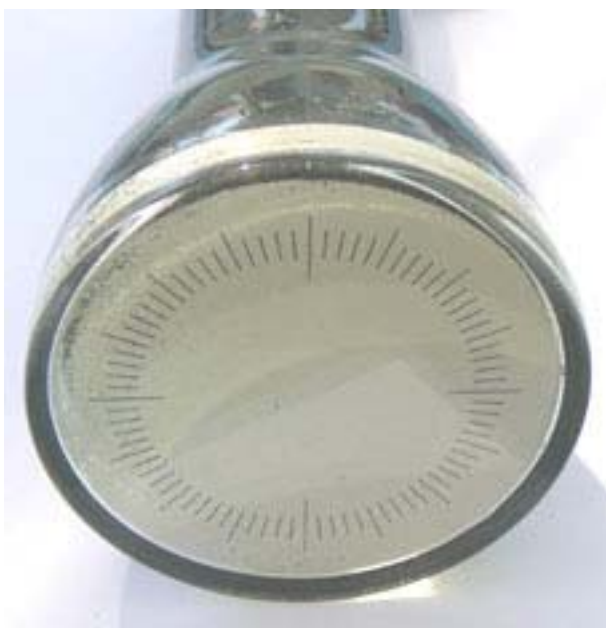
The Telefunken P07S1 CRT, left on the figure, was used as range tube on the indicator unit of the Lichtenstein FuG202 intercept radar.
