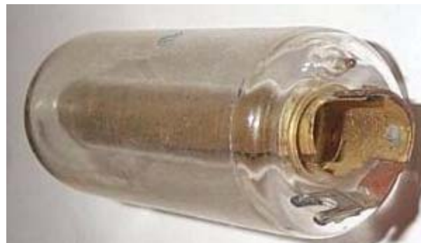
LG 75 Nullode with removed spray shield
