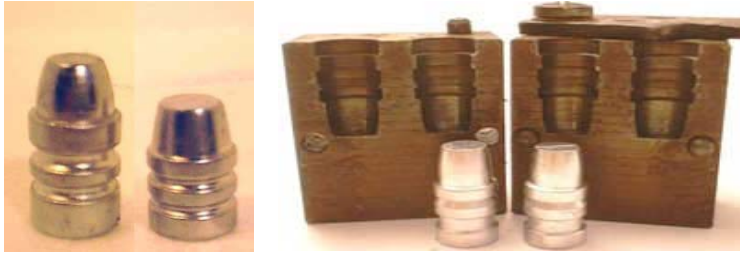
Early revolver bullet designs did not include a dedicated crimp groove (e.g. the Ideal 360271 and 360345 target bullets shown at left). Elmer Keith integrated a beveled crimp groove into the Ideal/Lyman 358429 (right) and most revolver bullets designed since then have followed suit.
