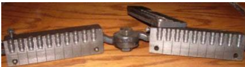
A well-used Hensley & Gibbs 10-cavity #51BB .38 semi-wadcutter mould (note the particularly massive sprue plate).
