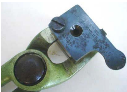
A single-cavity Herter's .38/.357 SWC mould cut by Lyman, with a 358156 cavity, with the Herter's sprue plate.
