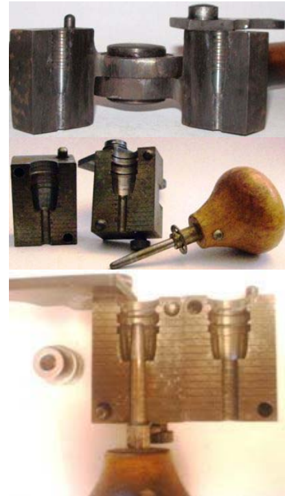
Early Ideal HP moulds had no "keepers" to hold the HP pin in (e.g. the old Ideal 25727 mould shown (top)). After 1940, Lyman HP moulds had keeper pins to hold the HP pin in place (e.g. the 454424 HP mould shown (bottom)), and after about 1990 they used a snap-ring to hold the pin in place (e.g. the 429244 HP mould shown (center)).
