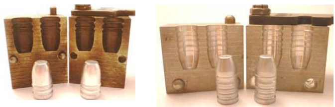
Some of the early cast bullet designs had relatively little bearing surface (e.g. the Ideal 403168). Designs with more bearing surface (e.g. the SSK 44 320 TC) are generally easier to get to shoot accurately.
