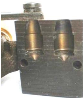
The Harvey Prot-X-Bore mould for the .38 SWC (Lyman 358502).
