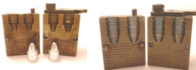
Originally Lyman's double-cavity detachable mould blocks were unvented, just like all the early single-cavity moulds (e.g. the Ideal 360302 Himmelwright wadcutter mould shown). Later on the double-cavity mould blocks were vented by the factory (e.g. the Lyman 357443).
