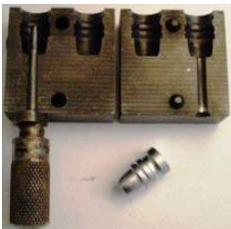
H&G #45 HP mould for the .44 Special and Magnum.
