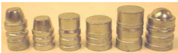
The wadcutter Class of 1905/1906 (l-r: Ideal 360271, 360345, 360344, 429348, 429352 and 452309)
