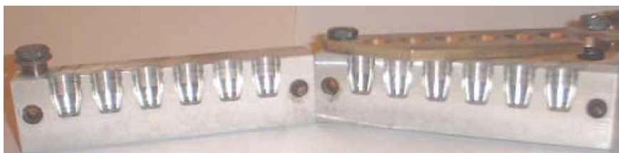
Lee 6-cavity .45 ACP TC mould.
