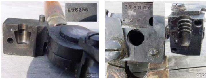
An example of a 2-part bullet (Ideal 375296). The small mushroom-shaped tip would be cast out of a soft alloy (like pure lead), then that piece would be inserted into the regular cavity of the bullet mould and the remainder of the bullet would be cast of somewhat harder alloy.
