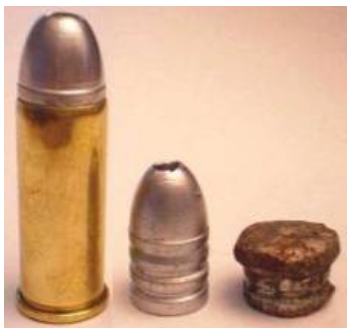
Excellent expansion and penetration from the 429251 HP at 1200 fps.
