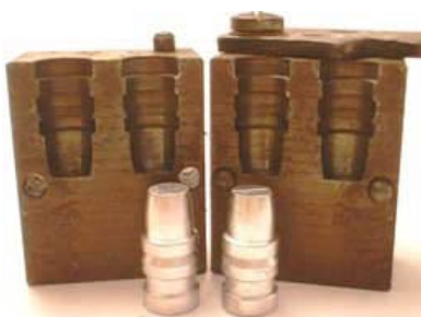
Elmer Keith designed the 358429 173 grain SWC for the .38 Special.
