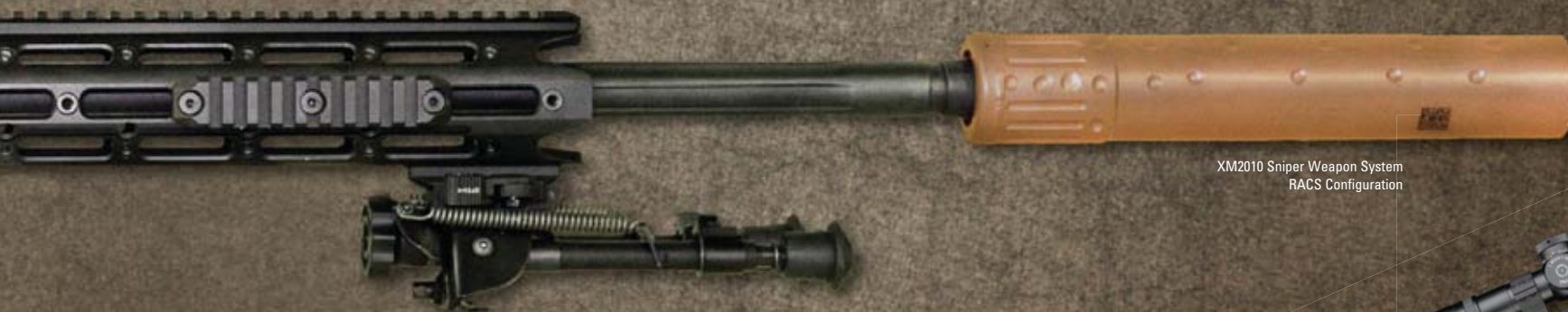
M24 SNIPER WEAPON SYSTEM » 24" 7.62 cold-hammer-forged 5R Rifling 416 stainless steel barrel • 1:11.25 twist • Composite aramid fiber-reinforced stock with aluminum bedding block • 5 round internal magazine • Leupold® Mark 4 M3 10x day optic • Steel rings and 2-piece base • Target-style iron sights • Deployment kit and hard case
