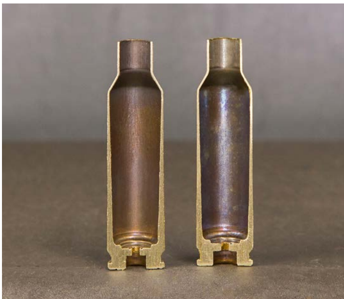
6.5 Creedmoor Starline Case cutaways with small (left) and large (right) primer pockets.
