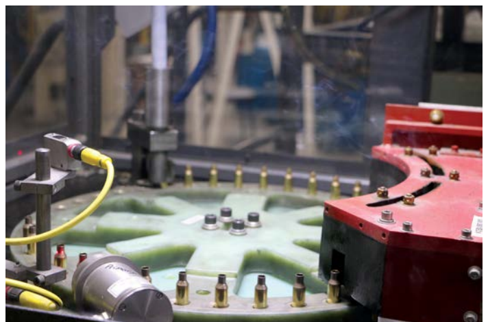
Induction neck annealing after forming and prior to final polish (Starline factory).
