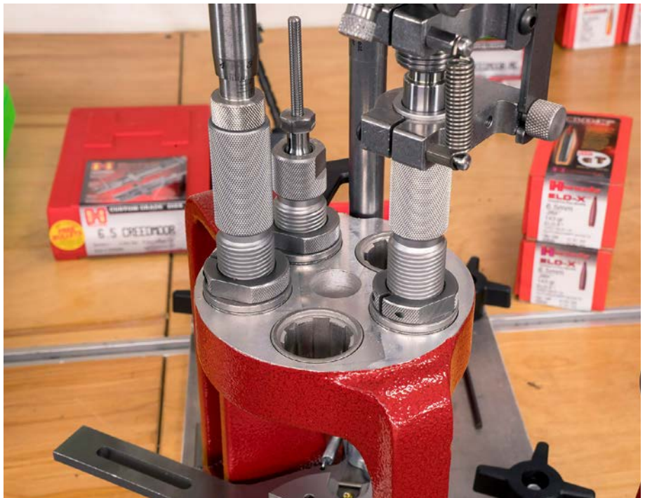
6.5 Creedmoor setup on the Hornady Lock-N-Load AP press.
