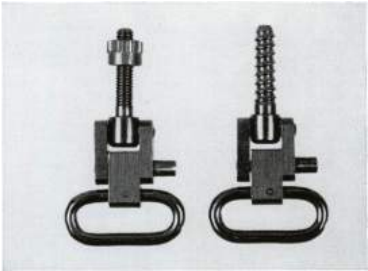
26 Fore-end swivel (1.) should be located 16" forward of trigger; buttstock swivel about 3 1/4" forward of stock toe. Screw hole for buttstock swivel is drilled at right angle to bottom line of stock. Hole for fore-end swivel must be counterbored for escutcheon nut, which should be tight drive fit in counterbore and must lie well below barrel channel lest it touch barrel.
