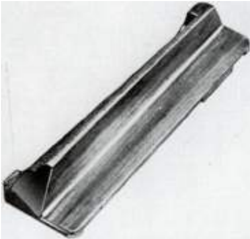
24 Rib of magazine follower is bevel-ground as shown so that the bolt will over-ride the follower when magazine is empty. The ground surface should be stoned smooth to reduce friction between bolt and follower.
