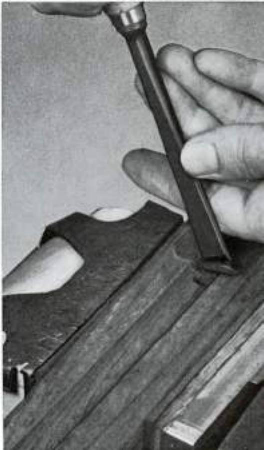
8 Initial step in inletting barreled action assembly is truing of receiver recoil shoulder in the stock. Flat chisel is used with paring motion to obtain absolutely flat surface. Very little wood is removed in this operation, but rounded corners left by stock inletting machine must be trimmed out to insure full contact of receiver recoil lug with matching shoulder in stock.
